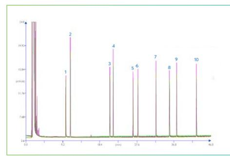
Purple trace: 5 different batches of capillary tubing
